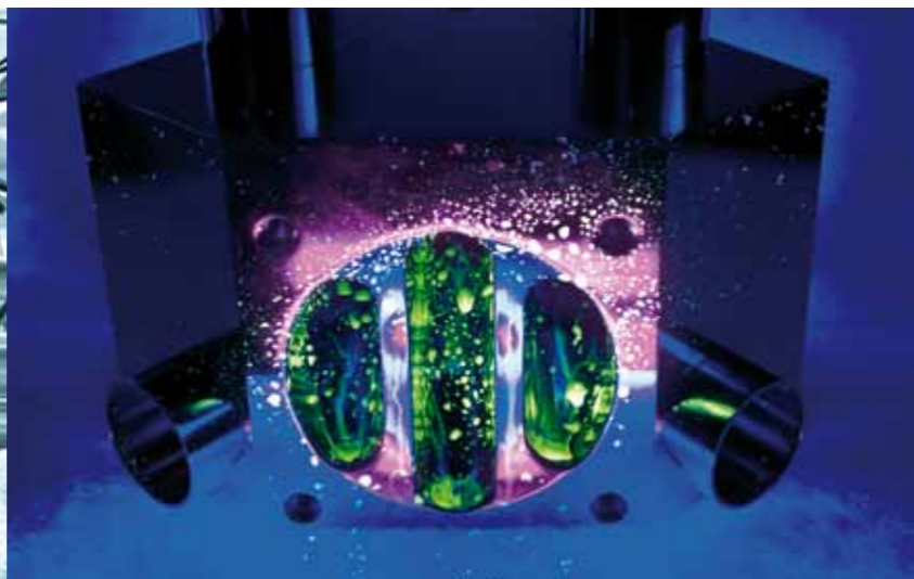
Visualization of the fluorescent effect of riboflavin under UV light in a valve interface
