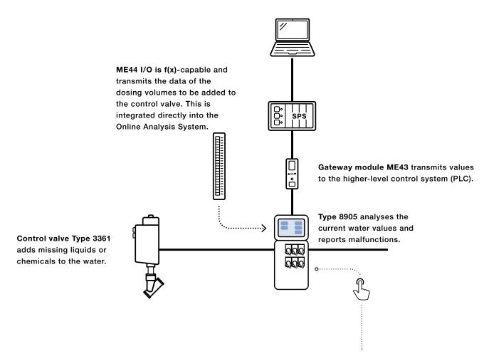
The configuration software "Bürkert Communicator" serves for parameterisation and diagnostic functions of the Online Analysis System. Cyclical values can easily be identified and displayed graphically. The f(x) graphical programming makes it possible to modify processes locally and individually without the need to intervene in the process control system.
